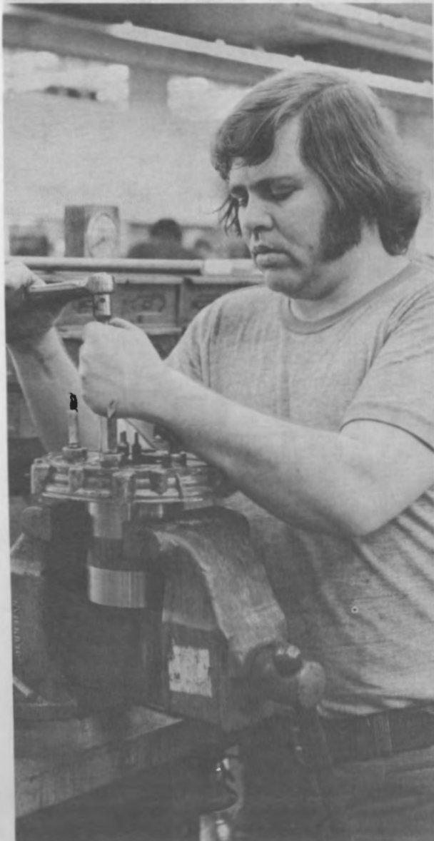
Joseph F. Cassell overhauls an oil-cooled generator, which provides the current needed to charge bus batteries.
