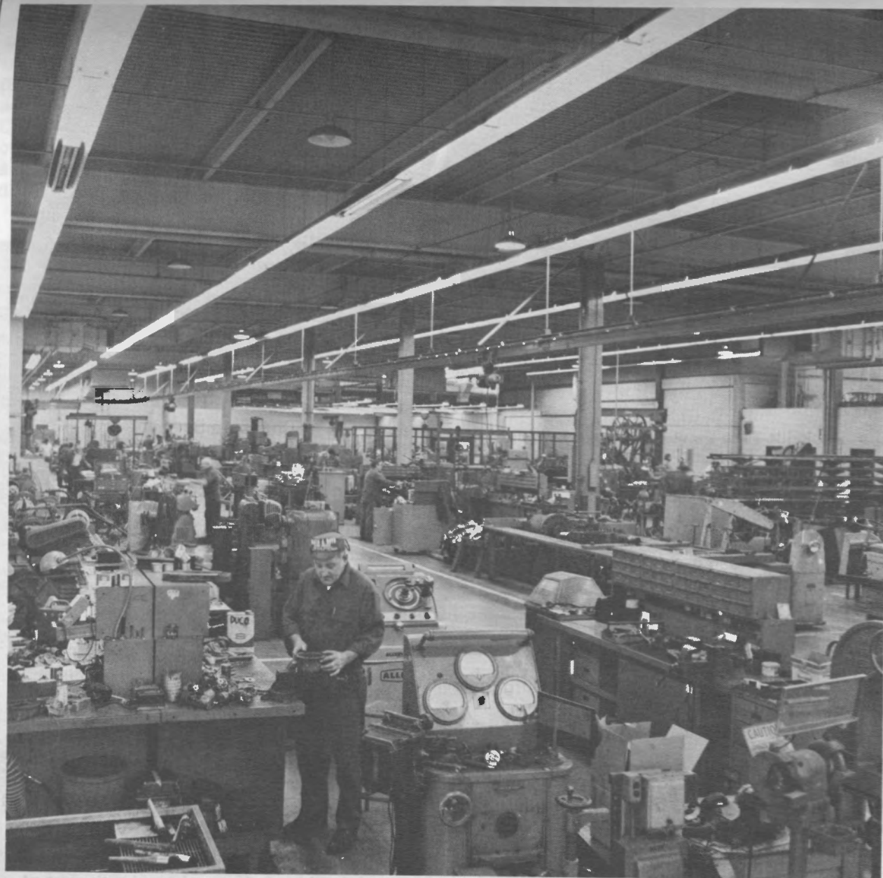
Seen here is a portion of WMATA's bus shop. Overall, the shop encloses an area equal to more than two-and-a-half football fields. The small units shop, which overhauls bus parts for later use as replacement, is in the foreground. The machine shop is in the background.
