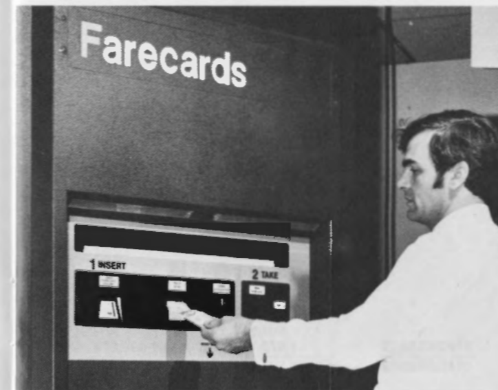
Passages leading to station mezzanines will contain fare-vending and change-making machines. Farecards will be used for exit as well as entry.
