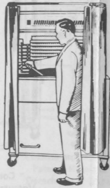
Voter moving the Red Operating Lever to the Right to Close Curtains
